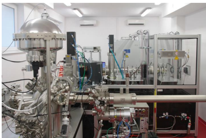
Fig. 3. Accelerator set-up for low-energy nuclear reactions at eLBRUS laboratories, University of Szczecin, Poland
